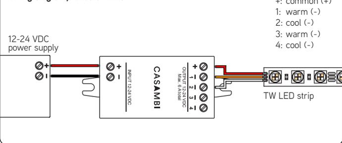
**Wiring diagram, 1-4 separate channels**
